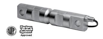
This product is designed for use in industrial and out-door environments. Nickel plated steel construction limits corrosion from outdoor use. The IP67 sealing makes it suitable for applications that are subject to high-pressure wash down. Tank weighing is made simple when this load cell is combined with the EZ mount mounting hardware it was designed for. Its high accuracy and availability in high capacities make it ideal for certified truck and rail scales.
